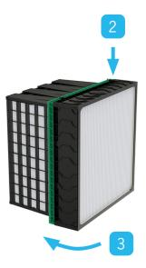
6. Lift the filter until the upper clips are released and remove the filter.
